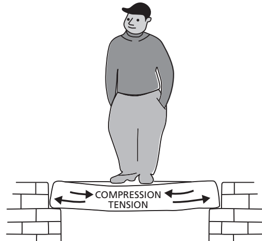
Figure 5.28 Stresses in a concrete lintel
